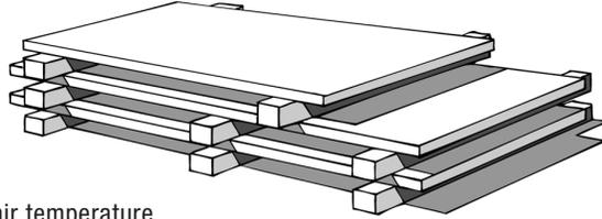
Constantly maintain indoor air temperature at 65-80°F and humidity at 50-60%. Shelf should be unpackaged and laid flat on spacers or otherwise positioned to allow air circulation to all sides for a period of time (preferably 24 hours) prior to installation.
