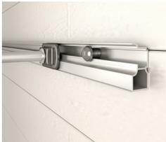
Attach the shelf pins to the rail with the provided bolts and nuts. Slide the nuts into the matching slot in the end of the rail. The set screw in the pin base must be facing downward. Then, attach the Rail to the wall with #12 pan-head screws.
