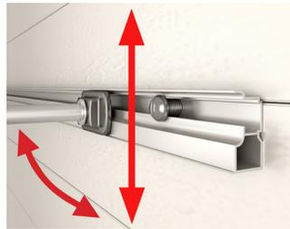
Adjust the pin angle by twisting the metal barrel of the pin – clockwise to raise and counterclockwise to lower. When the desired angle is achieved, tighten the set screw. You may prefer to level the shelves or to “pre-load” the angle upwards if a heavy load is expected.
