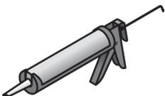
Use top-quality Silicone at sinks, joints, gaps at walls, etc. Never use construction adhesive with wood tops. We do not recommend using Silicone in lieu of install fasteners.
