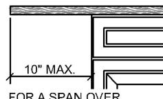
FOR A SPAN OVER 10", ADD A SUPPORT BRACKET
