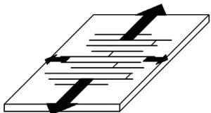
Wood worktops expand and contract front-to-back (across the grain). Allow expansion as shown above, or the worktop will crack.
