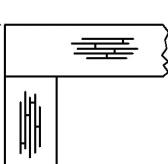
CaféCountertops custom tops are built to order with field joints typically factory-prepared for connecting bolts. Bolts should be snug but not over-tight. Tops without factory field joints may be rejoined by draw-bolts or connecting plates (not included). Fill gap with Silicone only. Do not use glue.
