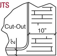
Cutouts located less than 10 inches from worktop end may cause cracking and will void product warranty. Seal all cut edges and inside faucet holes with Luxury Oil.
