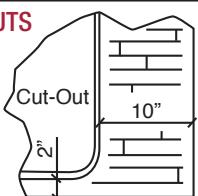
Cutouts located less than 10 inches from worktop end may cause cracking and will void product warranty. Seal all cut edges and inside faucet holes.
