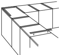
For best results in dry Rocky Mountain or northern climates, acclimate 48 hours. Install 1/8"-thick spacers between cabinets and countertop to permit air circulation to both sides of the countertop.
